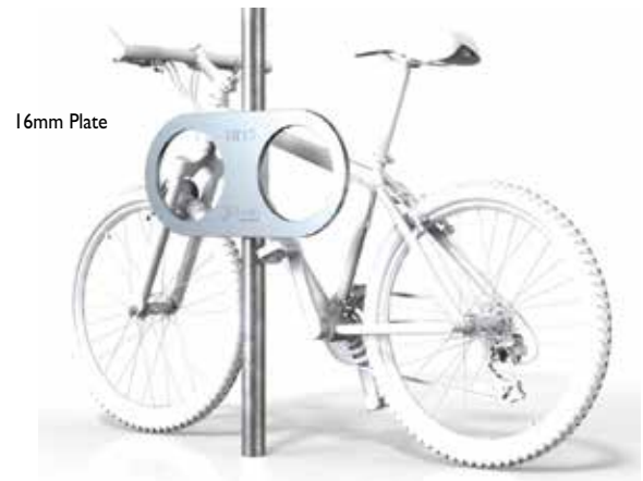
Units are designed to bolt-fix to existing 40NB or 50NB posts using M12 bolts & shear nuts
