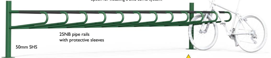
25NB pipe rails with protective sleeves
