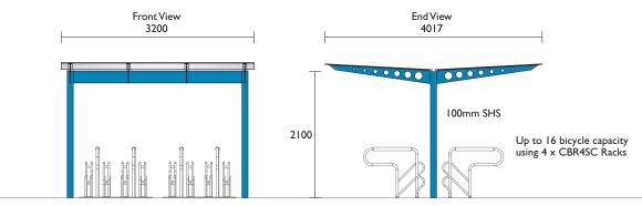
Material Specifications (General)Frame200 x 100mm U Section / 100 x 100mm SHS / Galvanised
